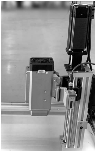
Fig. 7. Representation of the Z-axis with a rangefinder mounted.
